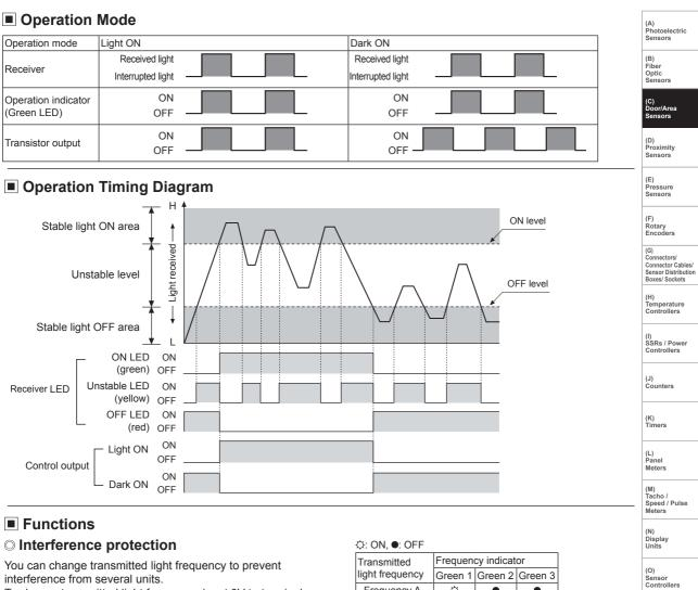
To change transmitted light frequency, input 0V to terminal 4 (black) MODE (for over 1 sec) of Emitter during normal operation.
