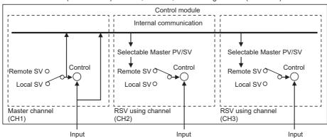
E.g.) RSV function is available when PV of TMHA (address 33, channel 1) is used for SV of TMH2(address 1, channel 3). Set RSV Master setting of TMH2. RSV Master address: 33, RSV Master channel: 1, RSV Master channel target: PV
