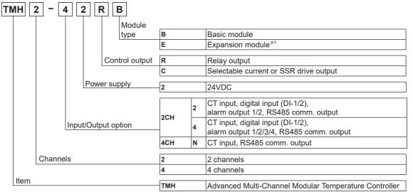
x 1: Since the expansion module is not supplied with power/comm. terminal. Order it with the basic module. €
