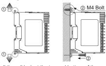
①Pull the rail lock at the top and bottom of the module. ②Insert bolts and fix it on rail lock. (fixing torque is 0.5 to 0.9N·m.)
