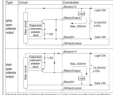
XIf short-circuit the control output terminal or supply current over the rated specification, normal control signal is not output due to the output short over current protection circuit.
