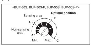
When place a target within sensing range of sensor, turn the VR from the minimum position and check the position 'A' where the operation indicator is turned on (Dark ON) or turned off (Light ON).
