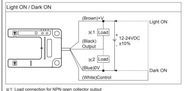
×2: Load connection for PNP open collector output
