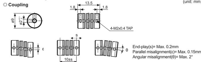
✗ When mounting the coupling to the encoder shaft, if there is combined misalignment (parallel, angular misalignment) between rotating encoder shaft and mate shaft, it may cause encoder and coupling's life cycle to shorten.
